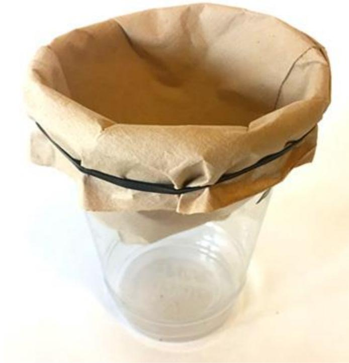
**Figure 5.** Using 4 layers of coffee filter, prepare a basket shaped filter inside each filtration cup and secure it with a rubber band.
