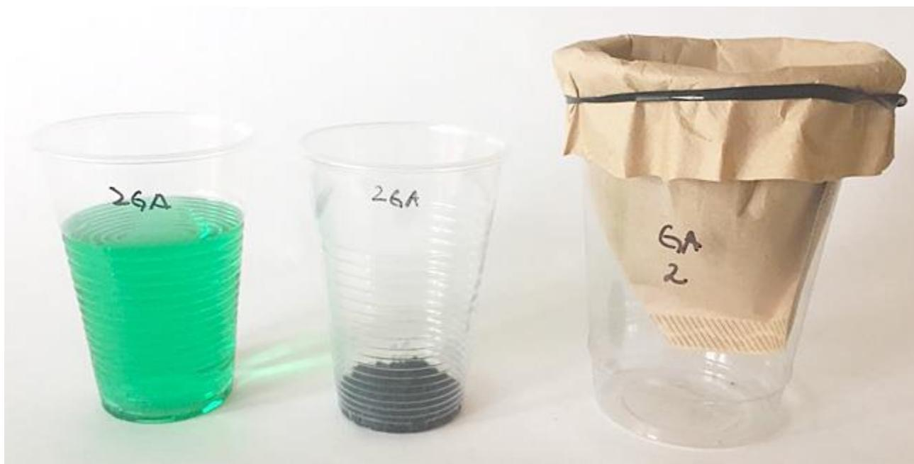
**Figure 6.** Arrange all prepared cups so that the colored water sample, the activated carbon and the filtration cup for each experimental condition and dye concentration are placed next to each other. In this image, the cups for the filtration experiment with a dye concentration of 2 drops per cup of liquid ("2") and granular activated carbon ("GA") are shown.
