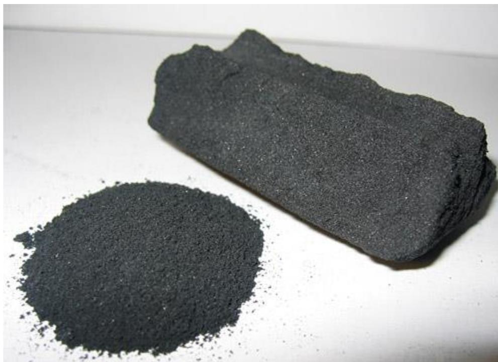
**Figure 1.** Activated carbon in powder and block form (Image credit: by Ravedave, via Wikimedia Commons)
