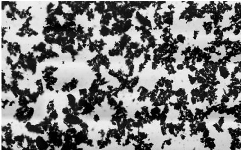
**Figure 2.** Activated charcoal particles viewed under a microscope (each particle is about 0.1 mm wide). The crumbly particle structure and shape result in a large surface area for each particle (Image credit: Zephyris, via Wikimedia Commons).
