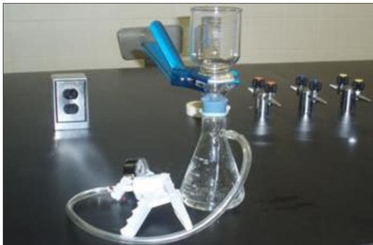
Figure 6. Apparatus for membrane filtration method
